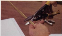
Brass miniature continuous hinges are a cinch to cut with a pair of metal shears. Make your cut at the joint where two hinge leaves meet nearest your ideal length.
