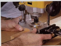
There are a variety of ways to cut the groove in the legs: A router table and a plow plane come to mind. I prefer to use a straight bit in a router with an edge guide. This allows me to see my cut at all times.
