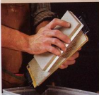
Norton waterstones and the DMT DuoSharp stone are a great combination. The DMT handles the grinding jobs and flattens the Norton waterstones (800-446-1119 or nortonabrasives.com ).
