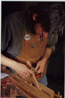
A spokeshave cleans up your saw cuts on the top rails quickly. After working with the fancy Leigh jig, it's a relief to pick up a tool that's simpler than I am.
