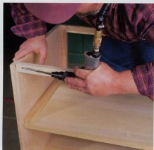
The bottom case uses a screw board to help support the top case and hold the back in place. Here I'm sawing the screw board to one of the bottom case's sides, flush to the inside edge of the rabbet.
