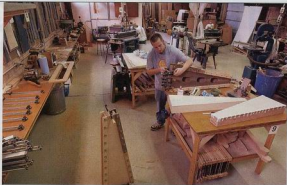
A broad view of the shop shows machinery staged along the right wall and back end of the shop. The finishing area is behind the wall in the back left corner. Benchtop machinery is staged along the counter that runs the entire length of the left wall. Assembly and workbenches are centered in the room and accessible from all sides.
