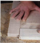
The door panels are held together with a cope-and-stick, and a loose mortise-and-tenon joint.
