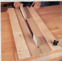
The gap between the fence bases on my dadoing jig represents the cut width. Finch scraps of the work material between them to set the jig.
