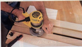
The gap between the fence bases on my dadoing jig represents the cut width. Finch scraps of the work material between them to set the jig.
