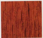
One of the disadvantages of a dye stain is that it doesn't get into the pores of open-grained wood, such as this piece of red oak.
