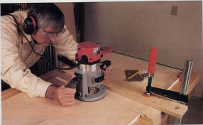
A crossbar attached at right angles to a plywood straightedge makes it an easy-to-align T-square guide for dadoing with a router. Clamp it securely to the work and the benchtop at each end.
