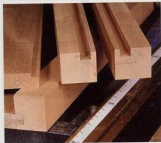
When your grooves and tongues are complete, they should fit snugly as shown. If you're not up to this task, you could simply glue the panel to the legs without any joinery. Just make sure you keep everything lined up so you're certain you'll achieve a tight joint.
