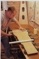
The sound box's backs finish out at 1/4" thick. To avoid lots of waste, the four-piece backs are resawn, then planed to 3/16", then edge glued. The special clamps (from Woodworkers Warehouse) allow Bryant Rees to make a thin-slab glue-up with reasonable ease.
